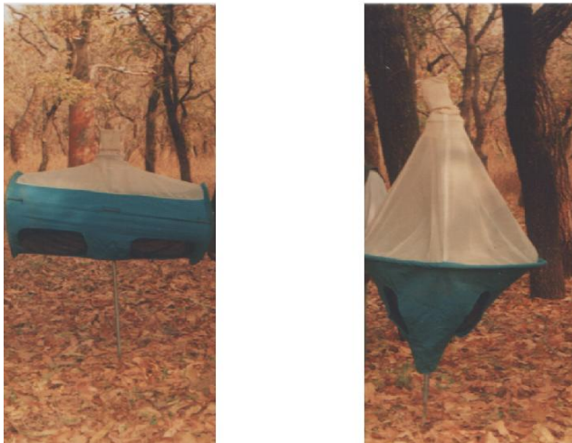
Figure 4. Drum-shaped and biconical-shaped traps for tsetse flies (Seifert, 1996).
