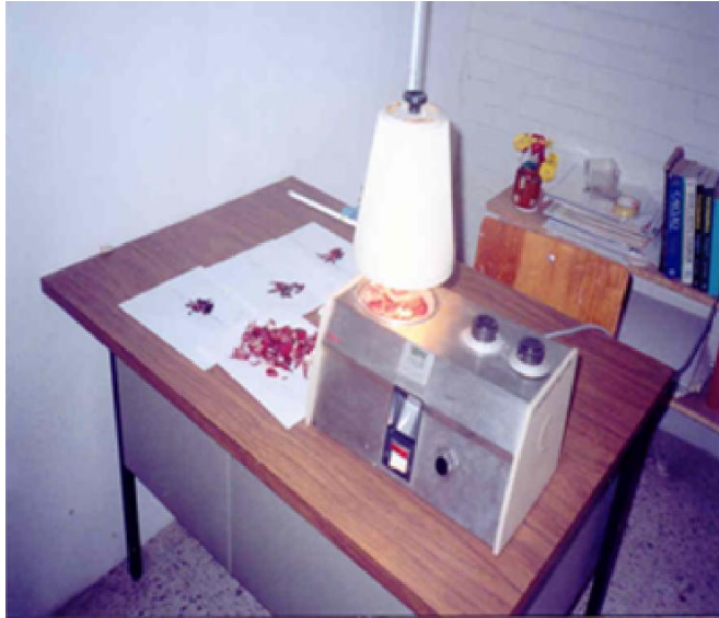
Figure 6. Determining Roselle drying properties using Thermobalance.
