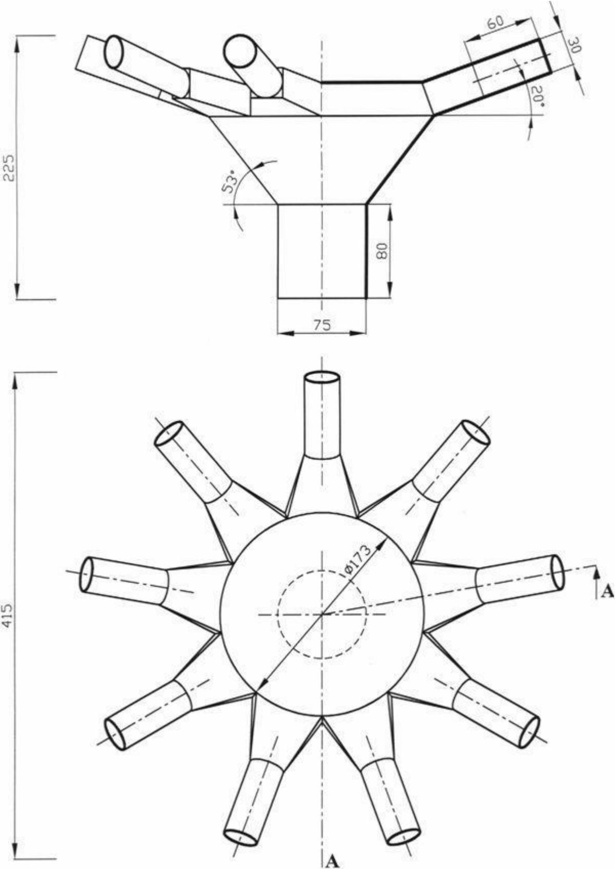
Figure 2b. Constructive properties of funnel distributor head.
