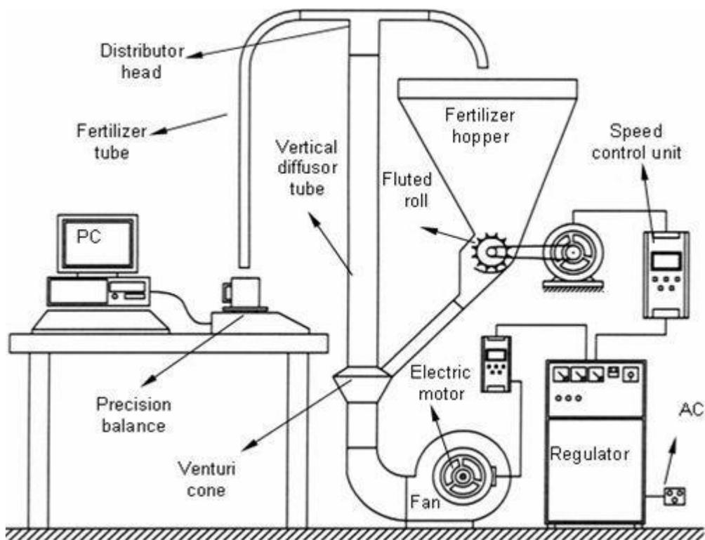
Figure 1. Measurement setup.
