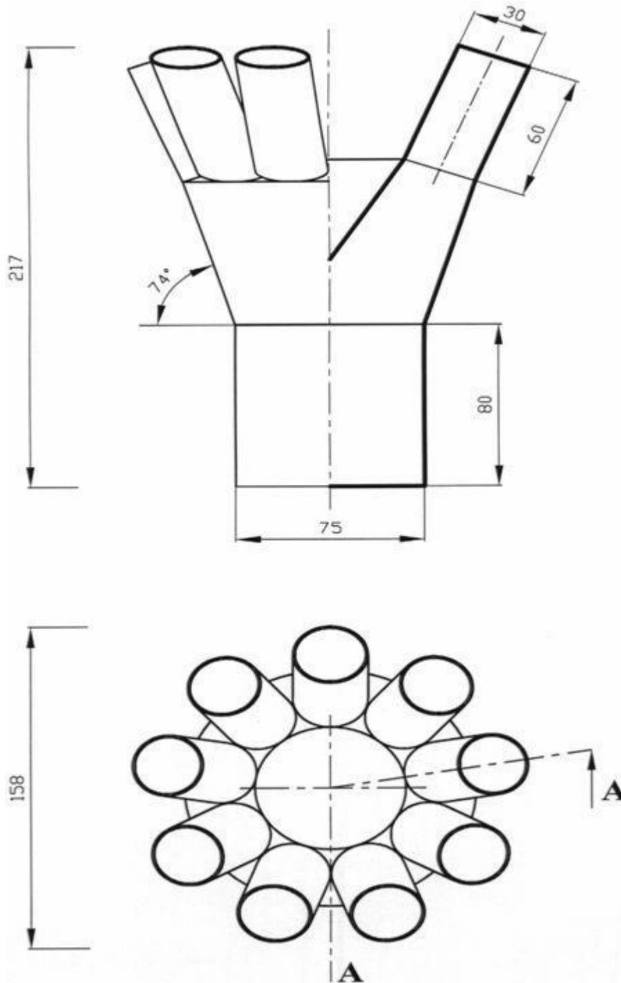
**Figure 2c.** Constructive properties of Y distributor head.
