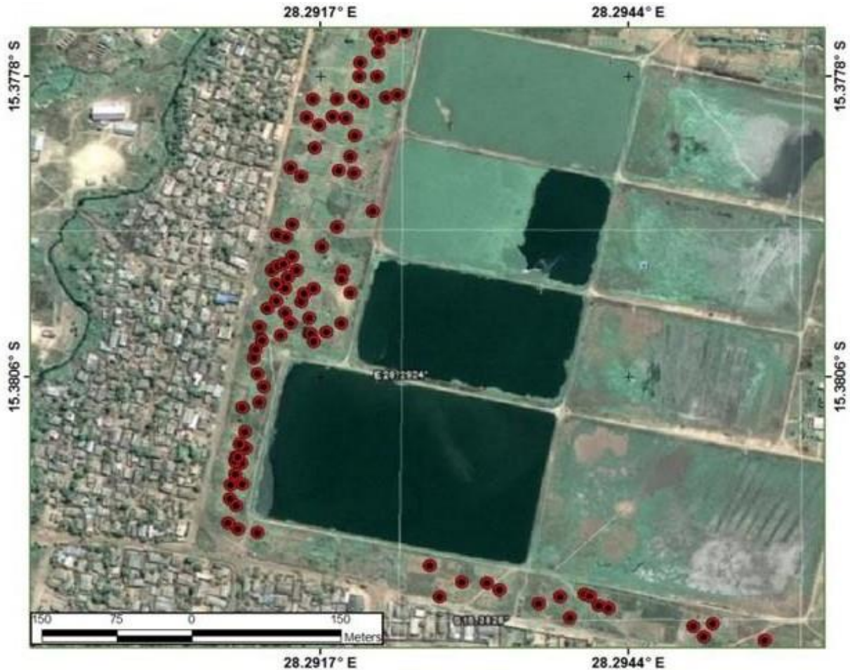
Figure 1. The scatter of shallow wells in vegetable gardens within maturation sewer ponds. Source: Google Earth Maps.
