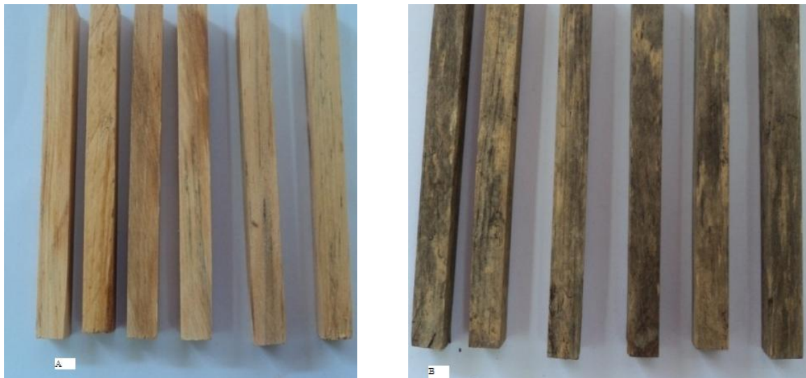
Figure 4. P. patula wood blocks A) before and B) after exposure to the tropical fungus in a soil bed test.
