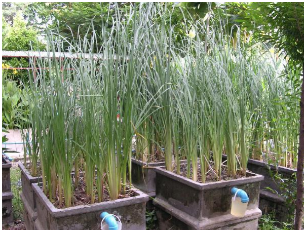
Figure 1. Flow diagram and photograph of the complete set of up-flow constructed wetland (UFCW) system
