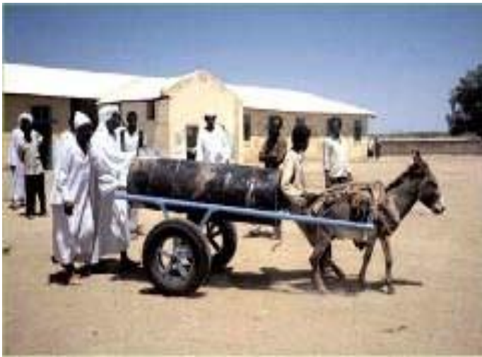
Figure 3. A typical donkey-drawn water tank used by water vendors.
