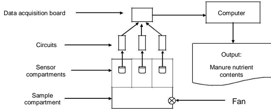
Figure 1. Schematic representation of the gas sensor array.
